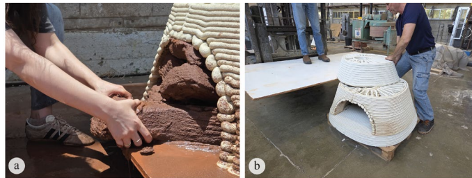
Figure 10. Assembly process. Mold dissolved in water (a); stacking segments (b)
