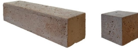
Figure 1. Cast beams and cubes for flexural and compressive strength tests
