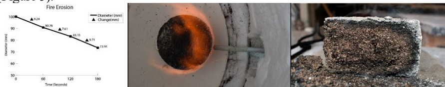
Figure 5. Left: Diameter change curve generated by experimental sample, demonstrating fire erosion behaviour. Middle: Experimental setup. Right: Result after 60 seconds exposure.
